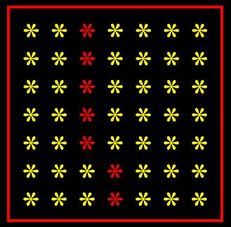
Up to 7 bits can be missed and there will still be only one error in each FEC block when the bits are read out row by row.
