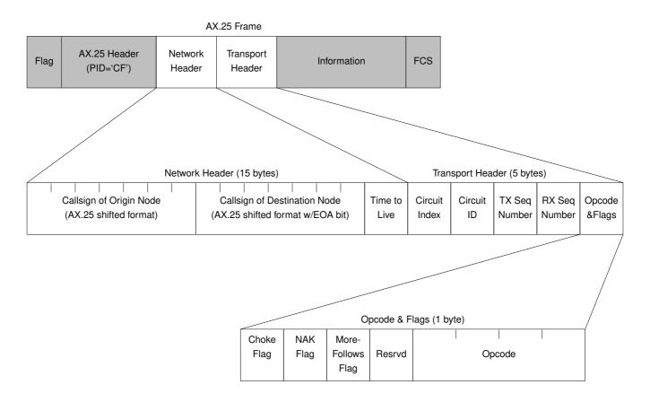
Each frame consists of a standard AX.25 link header, followed by a 15-byte network header and a 5-byte transport header. The network header contains the information needed for automatic routing, while the transport header supports end-to-end error and flow control for circuits.
